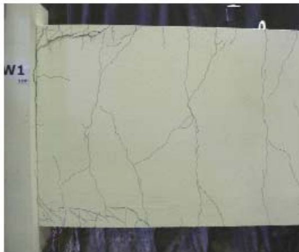
(c) photo at the end of testing Fig. 5. Response of Wall W1
