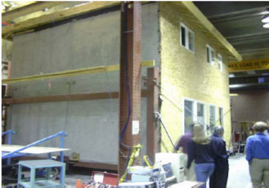
Figure 6. Full-scale wooden house on shake table for testing.
