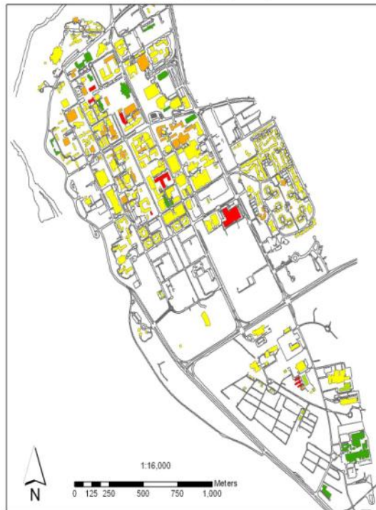
BC31 Mean Damage Factors with Modifiers Intensity IX - UBC Campus
