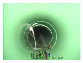
CCTV of Lateral to Property Line may identify this. Only 14% of surveyed municipalities are insisting on this CCTV inspection of the lateral (all through Push Camera launch from house basement)
