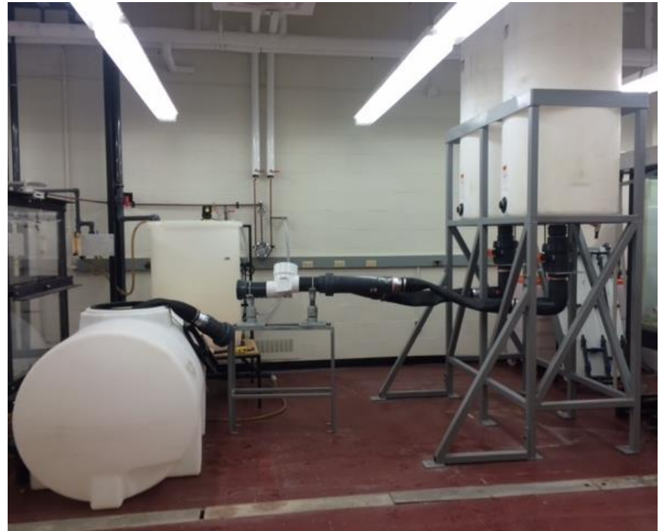
Constructed backwater valve laboratory apparatus
