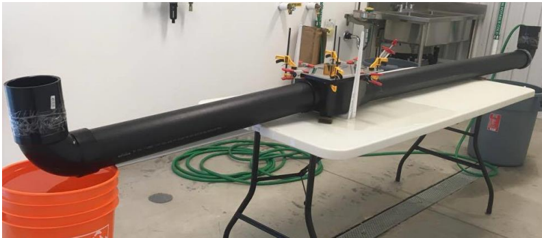
Laboratory model used to calibrate CFD model
