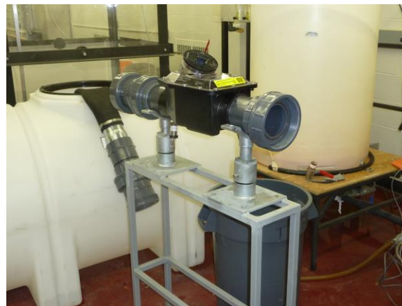
Laboratory model to test backwater valve performance
