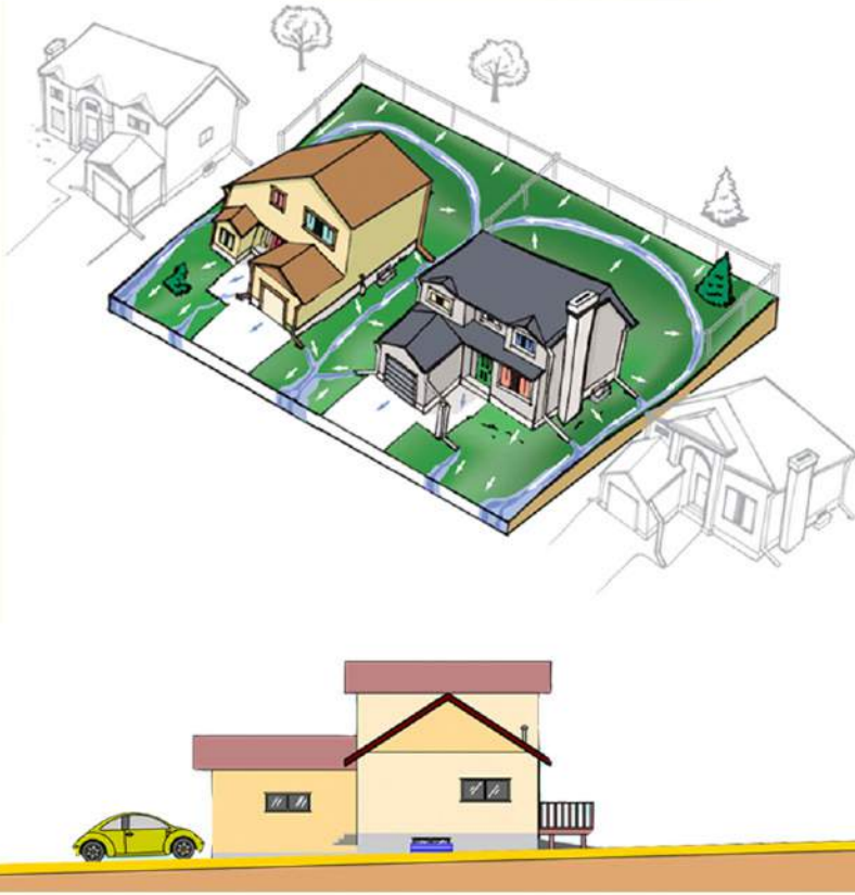
Figure 21 : The illustrations above were used by the City of Edmonton to show proper lot-grading. (Source: City of Edmonton)
