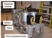
Figure 2: Pressure Load Actuator—The unit is about 600 mm wide and 1,200 long.
