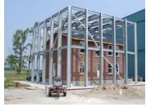
Figure 1: Full-scale house test specimen inside galvanized steel reaction frame.
