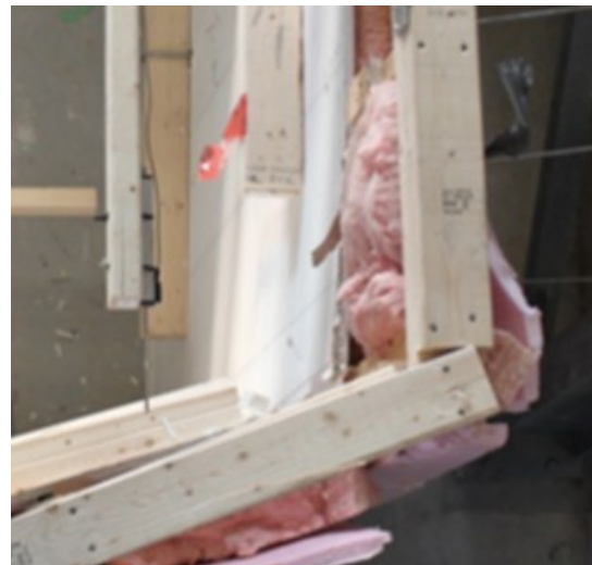
Photographs of corner displacements with brick cladding (left) and without bricks (right), at about the same load levels.
