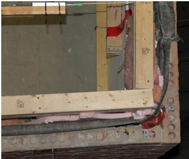
Photographs of corner displacements with brick cladding (left) and without bricks (right), at about the same load levels.
