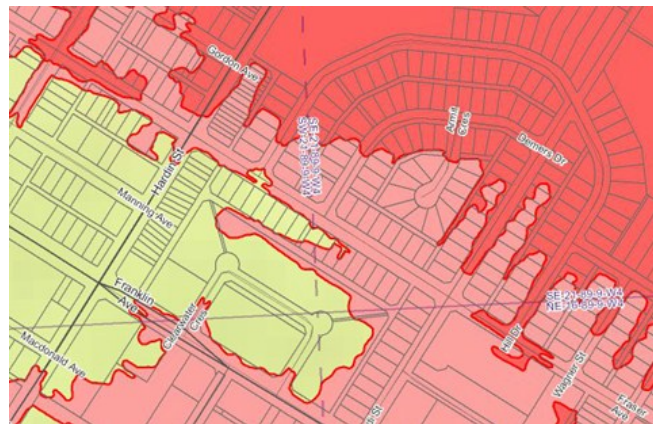
Figure 2: Zone Flood Hazard Area, Alberta. In Alberta, a two-zone flood hazard area is defined. Pink areas include the 1 in 100 year flood fringe, and red areas represent the floodway, where flood waters would reach at least 1 m in depth and flow 1 m/s during a 1 in 100 year flood. Source: http://www.envinfo.gov.ab.ca/FloodHazard/
