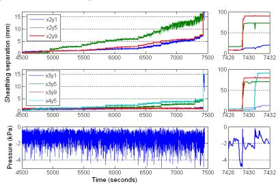
Incremental damage of sheathing fastened with twisted nails during a dynamic wind load test.
