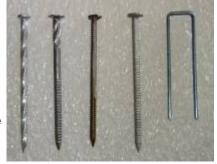
Photograph of the different nails used in the roof sheathing study. From left to right: twist-shank nail, HurriQuake® nail, adhesive coated ring-shank nail, another ring-shank nail, and a staple.
