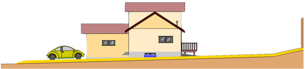
Figure 21 : The illustrations above were used by the City of Edmonton to show proper lot-grading. (Source: City of Edmonton)
