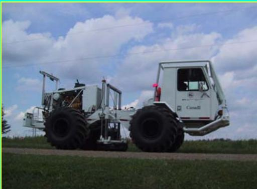
Shear wave reflection profiling.
