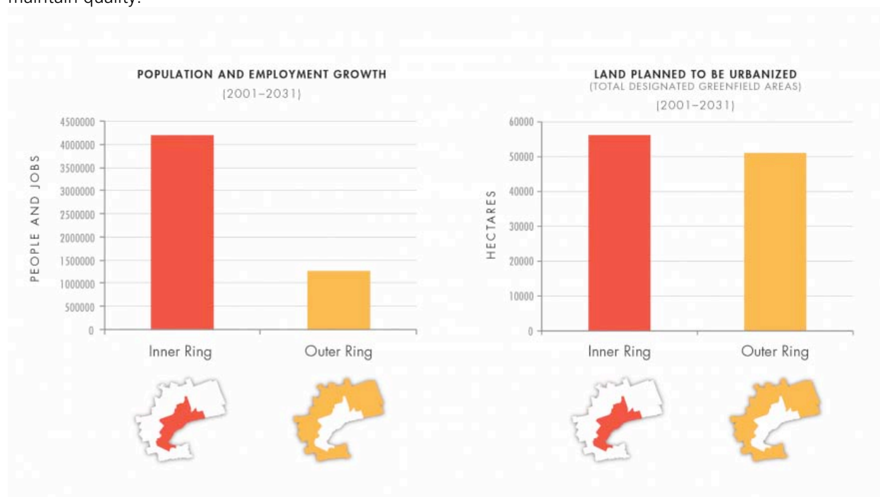
Figure 10. Low density development in the outer ring of the Greater Golden Horseshoe translates into more buried infrastructure per capita than in areas with higher development densities. Source: [Allen and Campsie, 2013.] 14
