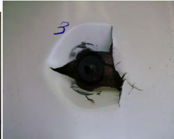
Crack patterns from PLA test
