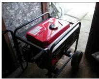
A generator was wired into the home's electrical service panel in order to provide power should a prolonged outage effect the area.
