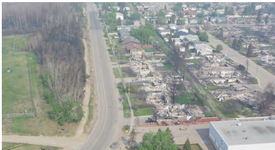
Figure 4-1: Typical separation of homes from forest fuel at Fort McMurray
