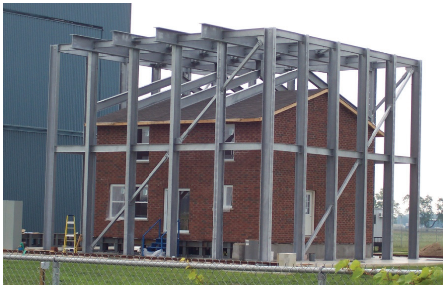
Figure 1 (right): Photograph of the two-storey test house at the Insurance Research Lab for Better Homes.
