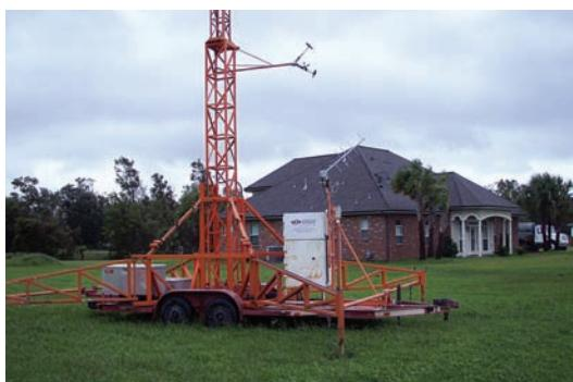
Photograph of tower belonging to the Florida Coastal Monitoring Program of the University of Florida, deployed in a suburban neighbourhood in Houma, Louisiana during Hurricane Gustav. This tower measured peak gust wind speeds of less than 80 mph. The house in the background was undam-
