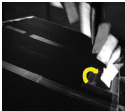
Close-up stroboscopic image showing a single realization of shingle flight from the roof of a house in a scale model wind tunnel study. In this image, the shingle fails in the lower right, gets caught up in high speed flow at the roof edge, and accelerates upwards, eventually moving downstream with a speed higher than the gust speed upstream of the house that actually caused the failure.
